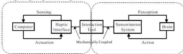
As illustrated in Fig. given above, haptic interaction occurs at an interaction tool of a haptic interface that mechanically couples two controlled dynamical systems: the haptic interface with a computer and the human user with a central nervous system. The two systems are exactly symmetrical in structure and information and they sense the environments, make decisions about control actions, and provide mechanical energies to the interaction tool through motions.
