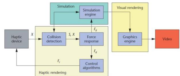
Haptic-rendering algorithms compute the correct interaction forces between the haptic interface representation inside the virtual environment and the virtual objects populating the environment. Moreover, haptic rendering algorithms ensure that the haptic device correctly renders such forces on the human operator. Several components compose typical haptic rendering algorithms. We identify three main blocks, illustrated in Figure shown
