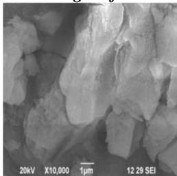
Figure 4b: SEM Images of ZrO2 nanoparticle
