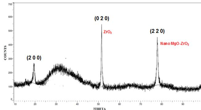
Fig.2. XRD pattern of MgO-ZrO<sub>2</sub> nanoparticles
