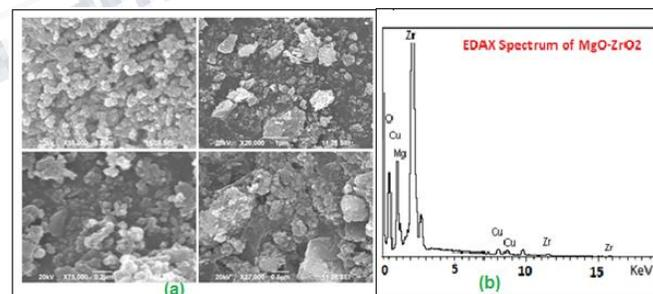
Fig 3(a). SEM image and (b) EDAX Spectrum of MgO-ZrO<sub>2</sub> nanoparticles
