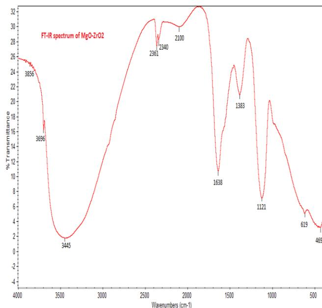
Fig.1. FTIR Spectrum of MgO-ZrO<sub>2</sub>
