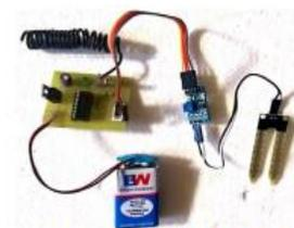
**Fig. 2 Remote Soil Moisture Monitor**
