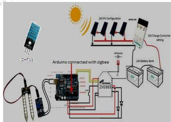
**Fig. 9 Remote sensing and monitoring system**
