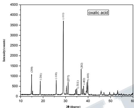
**Fig.2. Powder XRD pattern of oxalic acid**
