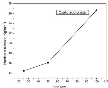
**Fig.6. Plot of hardness vs load**
