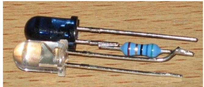
IR Sensors This sensor is a short range obstacle detector with no dead zone. It has a reasonably narrow detection area which can be increased using the dual version. Range can also be increased by increasing the power to the IR LEDs or adding more IR LEDs.
