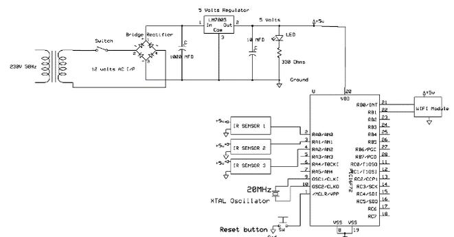
Our project “IOT based Smart parking system” is mainly intended to monitor the status of the devices through server (Wi-Fi).
