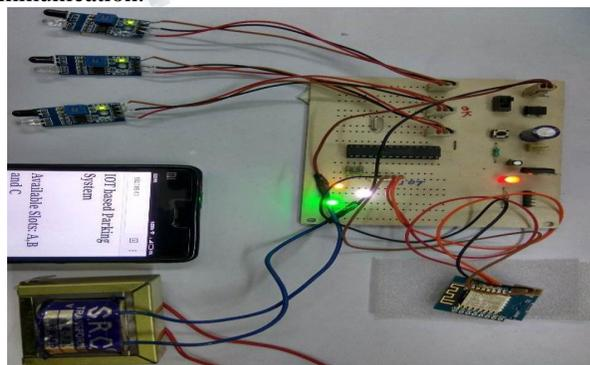
Fig.7. Working model of project In this system, the user has to be connected to the Wi-Fi network of that particular parking area through which he is given access to the webpage and can know about the status of the parking slot.
