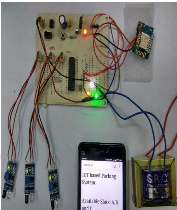
The project “IOT based Smart Parking system” was designed such that the status of parking slots can be known from anywhere in the users webpage. This is achieved using Wi-Fi communication.
