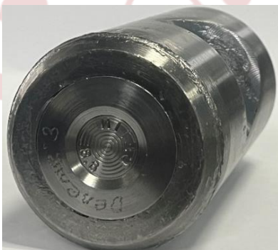
Figure 4. One of the marking dies that is placed inside the sleeve
