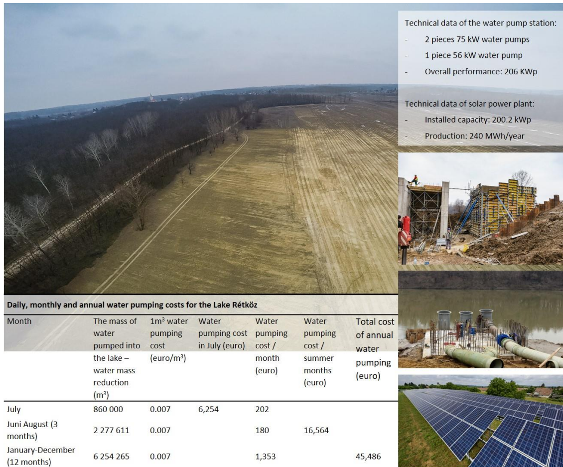
Figure 4. Dredging of the lake bed and the installation of a pumping station at the mouth of the inlet channel to the lake. The costs of maintaining the permanent water security of Lake Rétköz.
